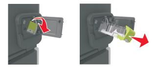
Use the metal tab to lift the staple guard, and then remove any loose staples.
