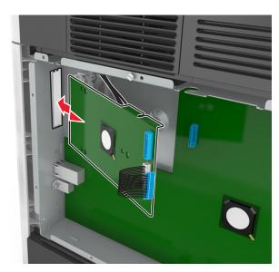
**Note:** Hold the ISP at an angle over the plastic bracket so that any overhanging connectors will pass through the ISP opening in the controller board cage.
