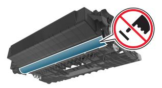
**6** Insert the imaging unit into the printer by aligning the arrows on the side rails of the imaging unit with the arrows on the side rails inside the printer.
