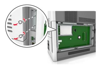
4 Remove the printer hard disk.
